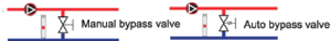
Figure 10 - System installed with bypass valve
